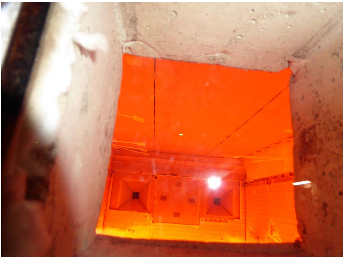
The fire exposed side after approx. 20 minutes of the test.
