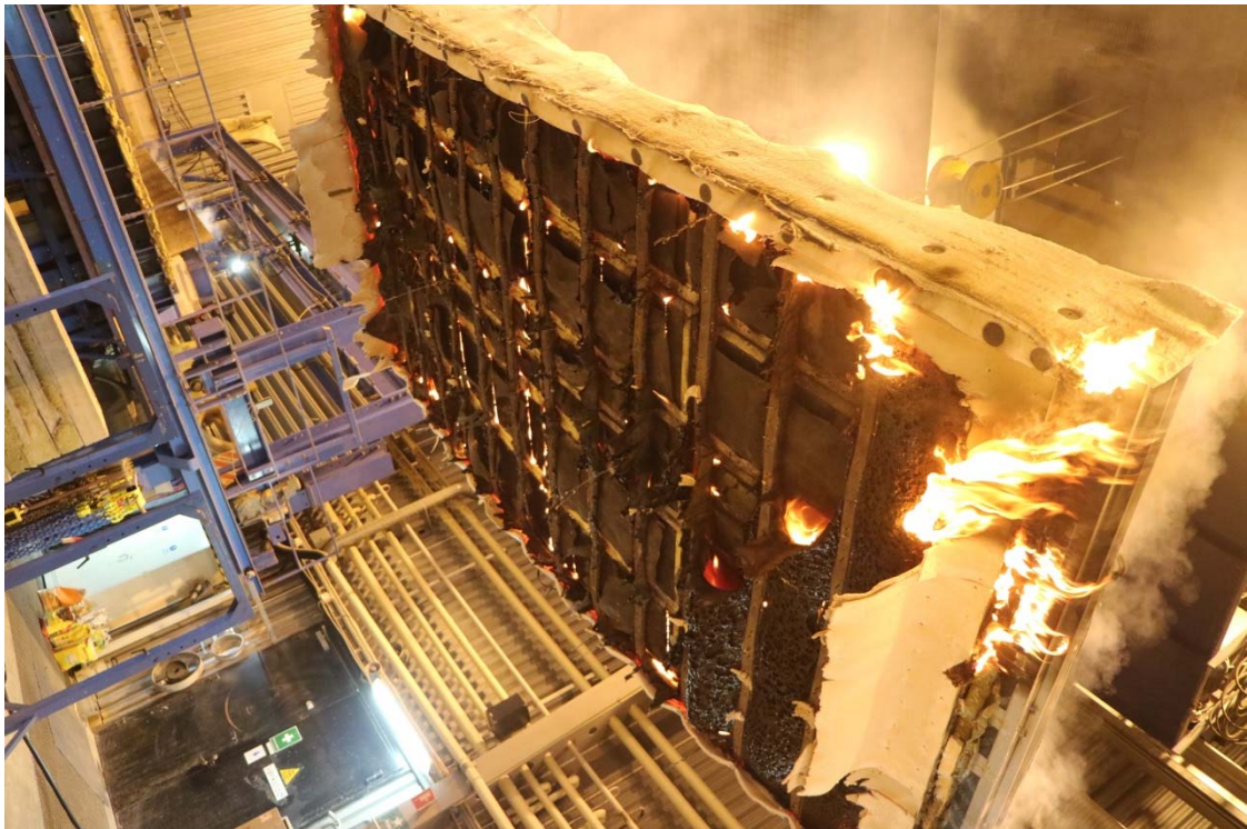
The fire exposed side of the test specimen after the test
